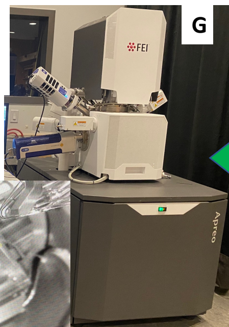
Thermo-Fisher Apreo 2 LoVac SEM with Oxford EDS and Oxford Symmetry 2 EBSD Detector
