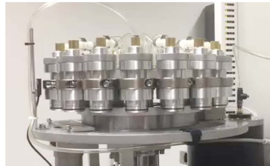
16-powder hopper allows for manufacturing of complex sample libraries
