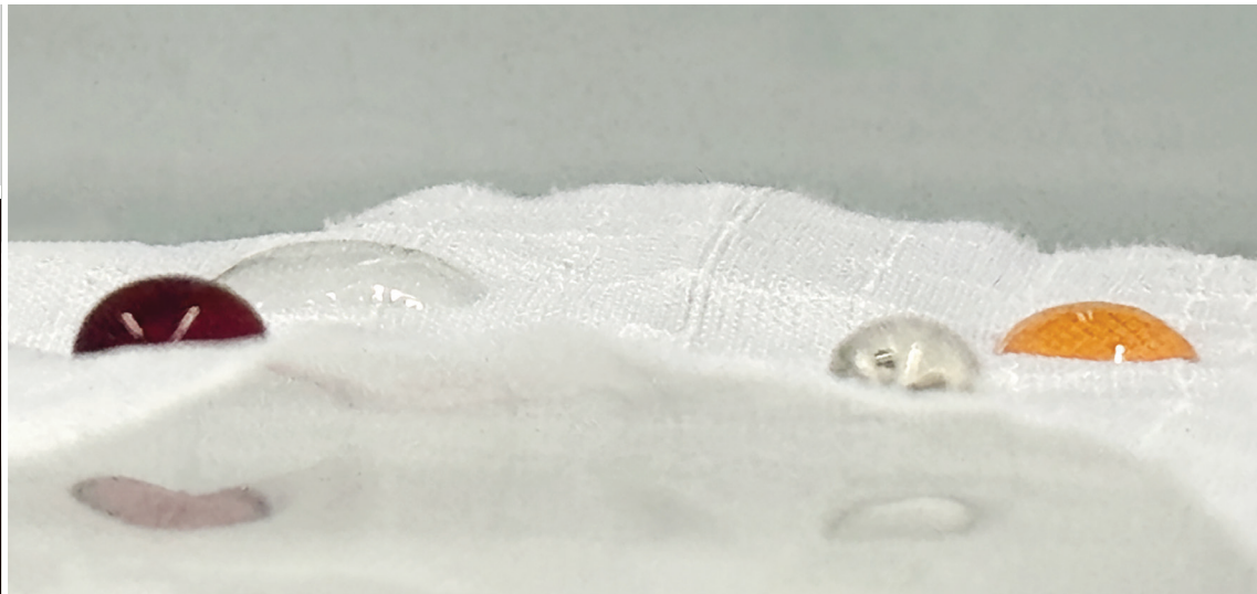
■ Figure 1. Nylon textile fabric treated with an omni-phobic P-silyl coating repels multiple liquids. Clockwise from lower left: wine (red), oil (clear), coolant (orange), and beer (yellow).
