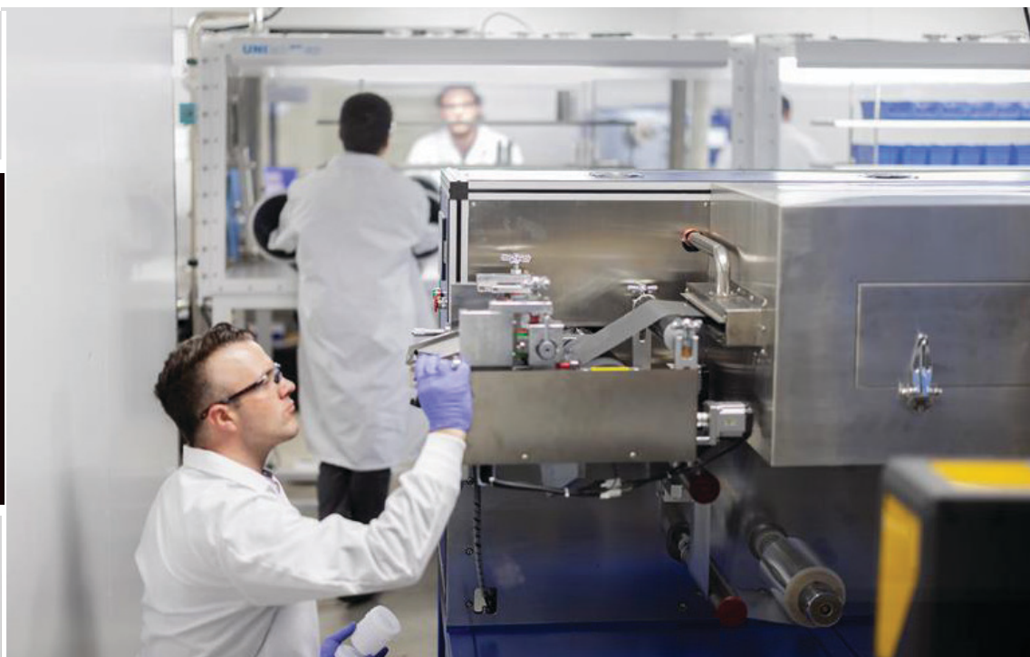
■ Figure 1. A researcher monitors hot-roll pressing of the thinnest, most scalable tape-cast solid-oxide electrolyte reported to date, producing a dense ~2- \mu m layer and fuel cells exceeding 4 x 4 inches.
