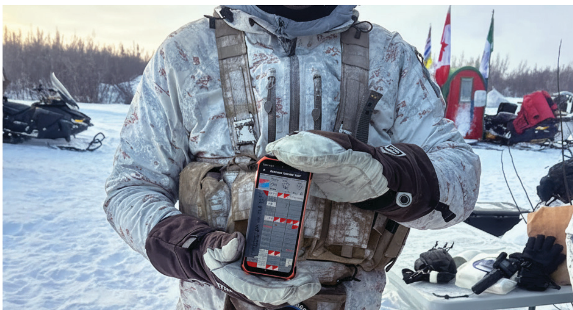
■ Figure 1. A Warfighter and his smartphone at Operation Musk Ox II. The phone is running an application that monitors all fiber computers for his unit (i.e., shirts, pants, boots, and gloves).
