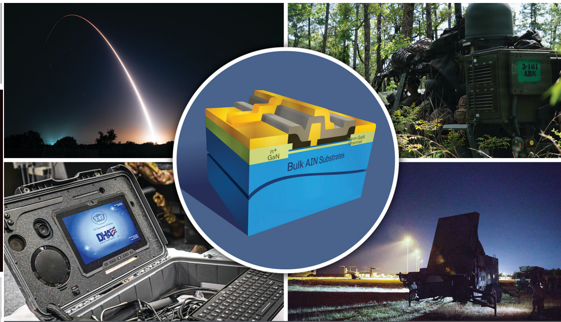
■ Figure 1. 3D representation of a fully fabricated XHEMT comprising a 500-nm AlN buffer layer grown on single-crystal AlN substrates, 20-nm GaN channel, and 6-nm AlN top barrier capped with a 1-nm GaN layer. The GaN channel layer is doped with silicon to prevent formation of positive charges at the bottom GaN/AlN interface and increase electron density in the channel.
