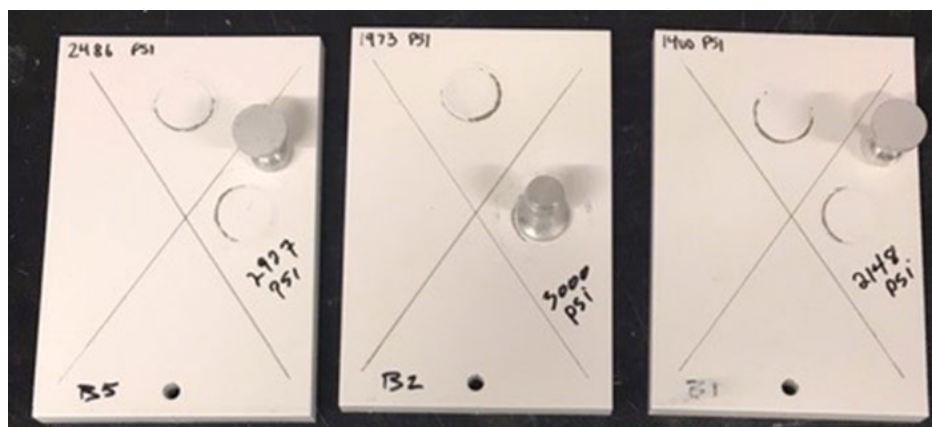
Fig. 8 Pull-off adhesion of postexposed Bonderite M-NT 7400 pretreated and MIL-DTL-53022 coated Ti test panels
