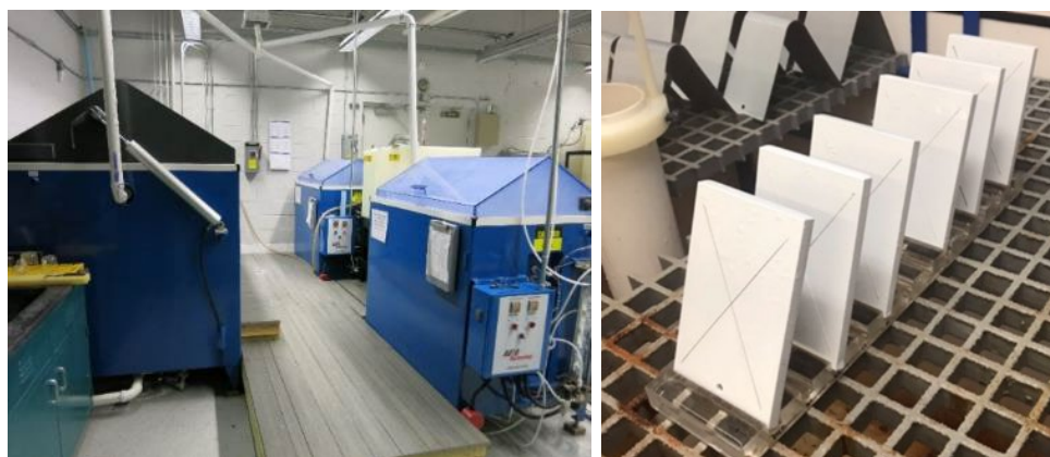
Fig. 2 Salt fog chambers (left) and coated and scribed Ti panels in chambers (right)
