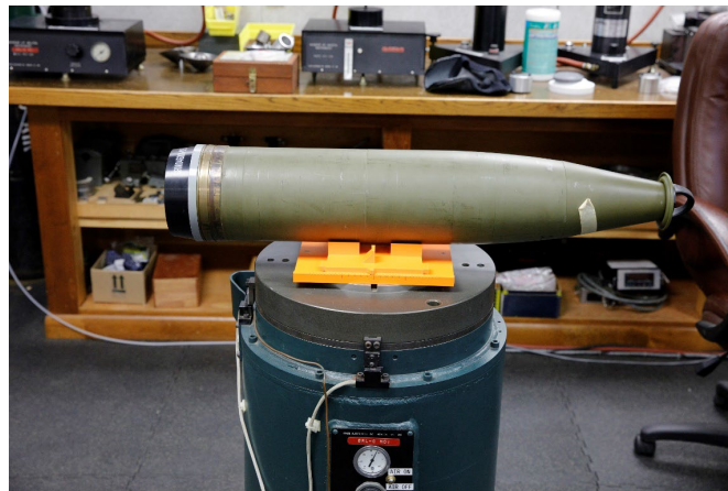
Figure 20. MOI-C with sliding fixture for large-caliber, with 155-mm projectile.
