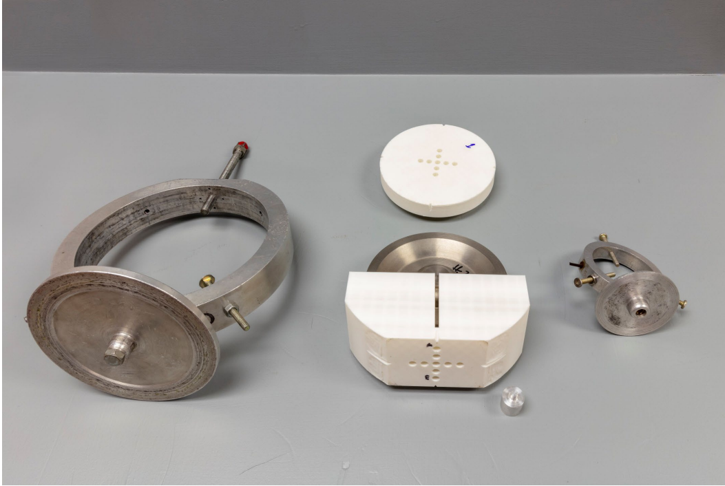
Figure 17. Various MOI-B fixtures.
