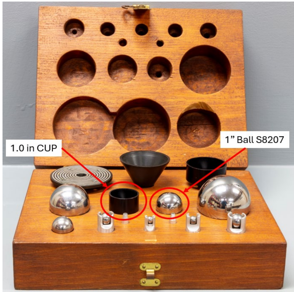
Figure 13. Calibration weights and mounting fixtures for MOI-A, MOI-AA, and MOI-AAA machines.
