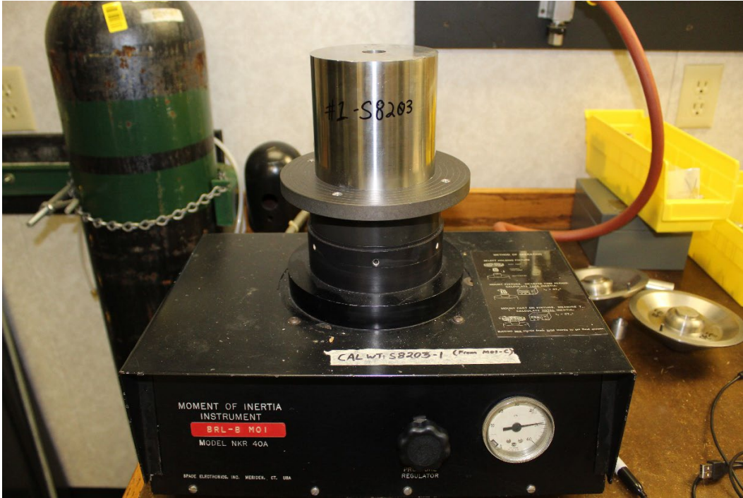
Figure 22. MOI-B with calibration weight.
