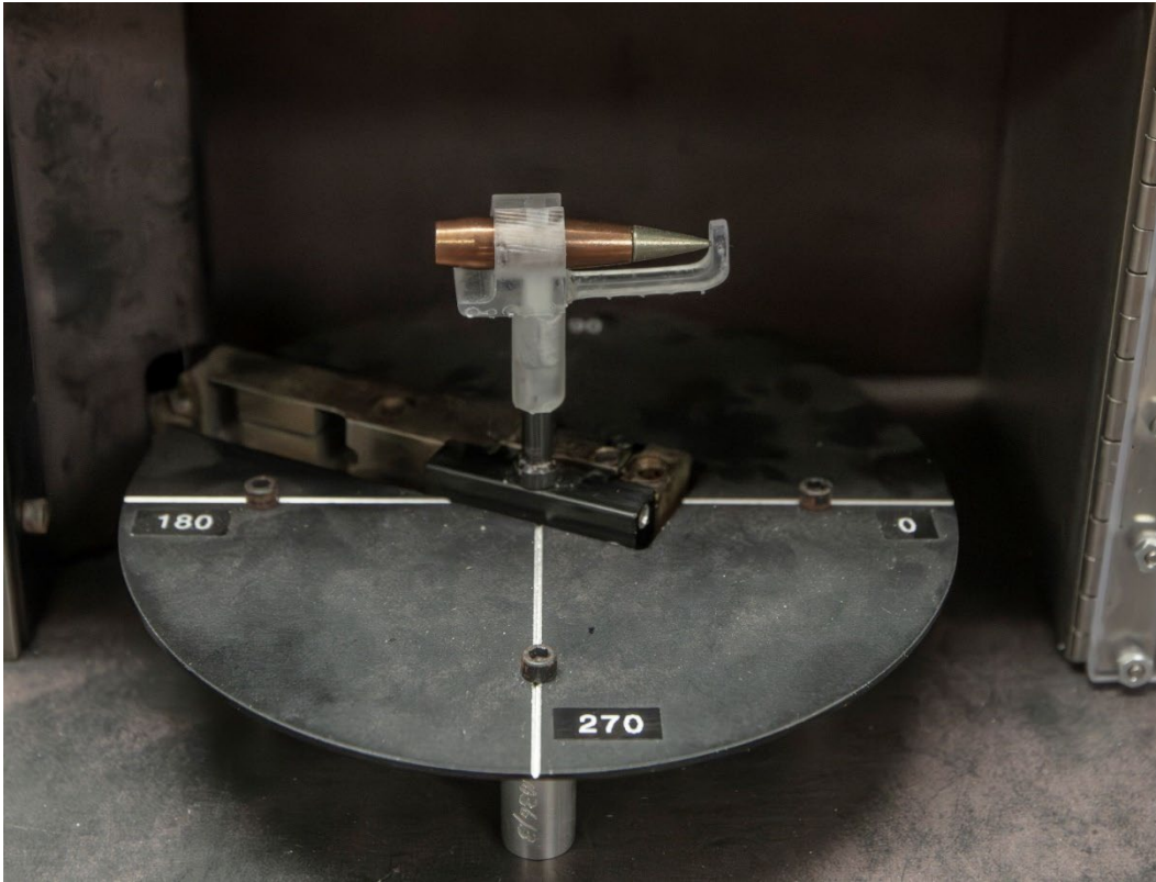
Figure 9. Fixture mounted on CG-A machine and oriented in the 0° position (fixture stop to the right).
