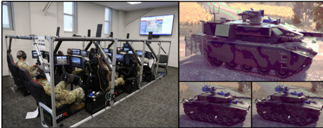
Figure ES-1. One configuration of ARL’s INFORMS Laboratory. The seven Soldier participants sitting in the wireframe simulator (left) are occupying an emulated future manned control vehicle (MCV) shown to the right (top). From front to back, a single vehicle commander sits in the lead position and gunner-driver pairs sit in the successive rearward rows to control the MCV, as well as two uncrewed robotic combat vehicles (right-bottom). Combined with a second wireframe simulator (not shown), doubling the simulated asset count to a section of six vehicles, this uniquely immersive mixed-reality simulator provided a high-fidelity operational space to safely explore advanced, yet experimental, next-generation systems in high-risk direct-combat scenarios, with appropriately trained and experienced operators.
