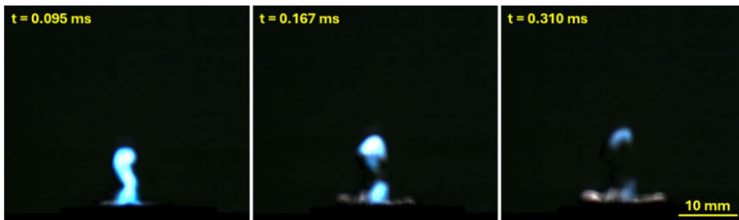
Figure 24. Example snapshots from a high-speed video of the post-plasma combustion for micron-sized aluminum.
