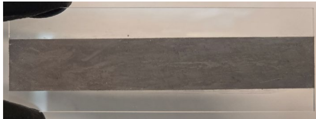
Figure 3. Example of proper sample preparation where the material has been evenly spread across the tape and the excess material been removed without leaving streak marks.
