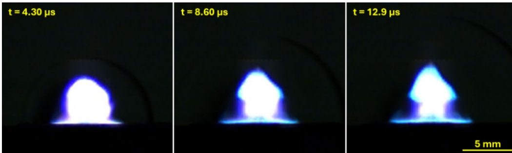
Figure 23. Example snapshots from a high-speed video of the laser-induced plasma for micron-sized aluminum.
