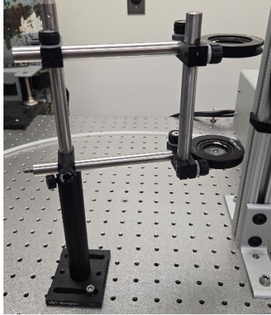
Figure 26. Two-iris setup used to align the vertical laser pathway.
