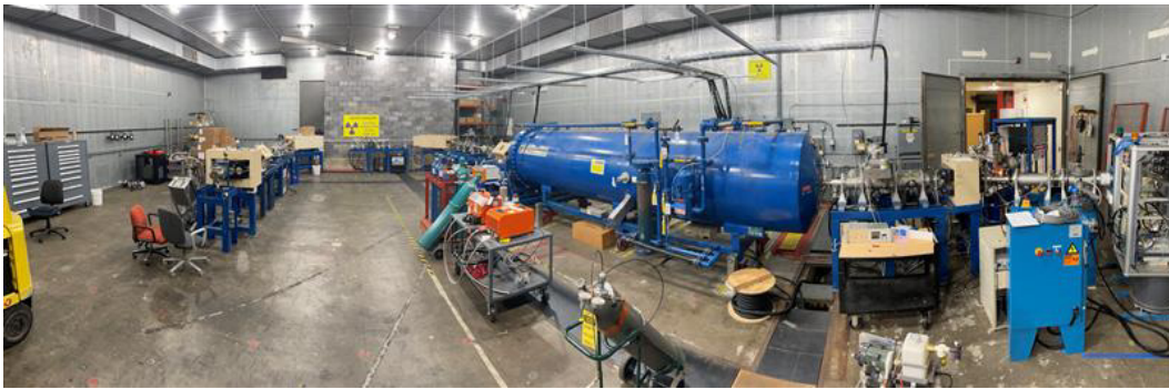
Fig. 1: The APEX facility showing the ion sources (grey) to the far right, accelerating tank (blue) center, and the target chamber (grey) to the left.
