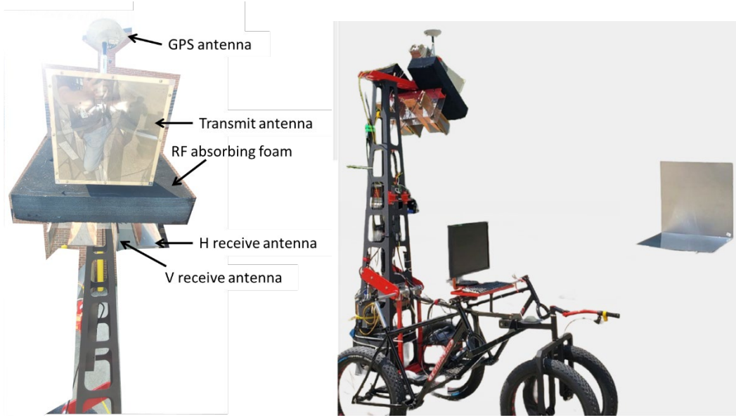
(a) Quad-ridge transmit and Vivaldi receive antennas. GPS data required for SAR image formation and in-scene calibration.
