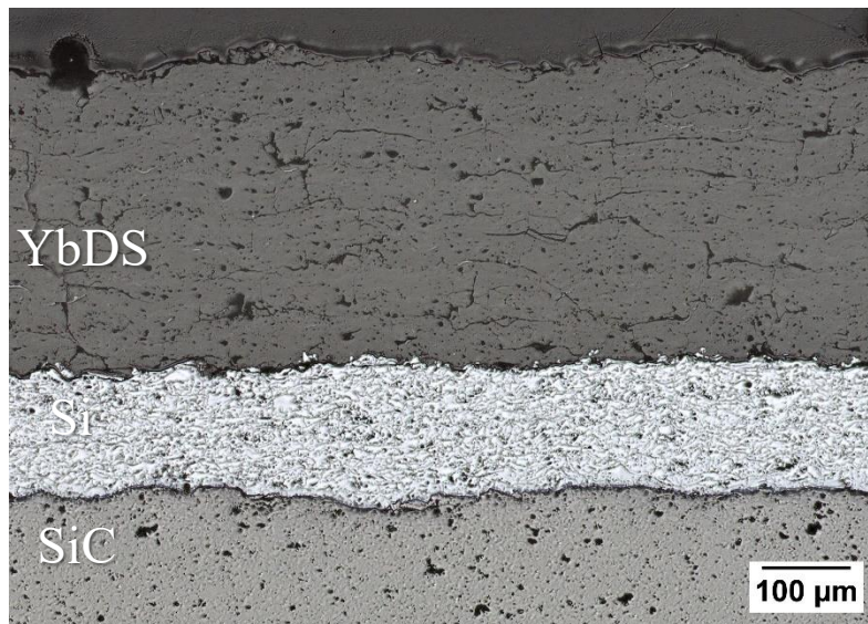
Figure 1. A representative image micrograph of a bilayer YbDS-Si coating on top of monolithic SiC substrate.
