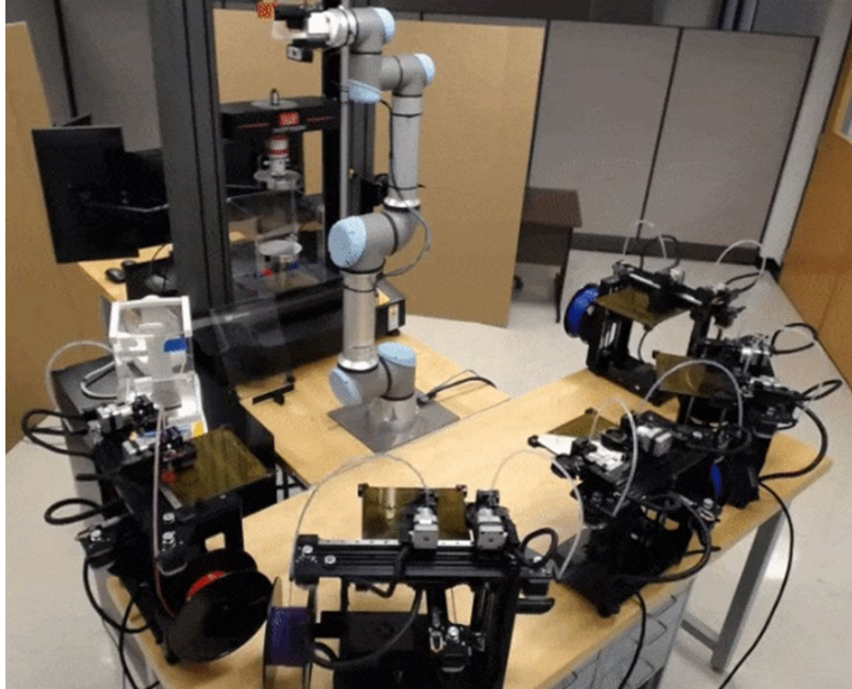
Figure 1. Reference image of self-driving laboratory including a mechanical load frame and 3D printer. Reprinted with permission from the automated mechanical test of Bayesian experimental autonomous researcher, Dr. Keith Brown, Boston University. 2
