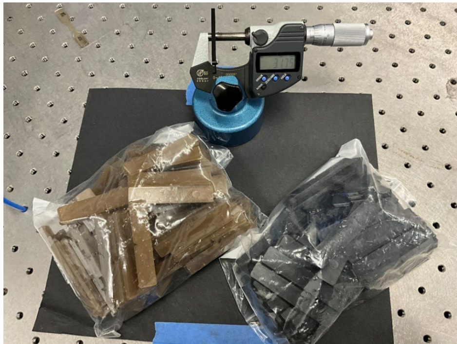
Figure 2. Large lots of injected molded test samples with manual micrometer measurement gage.
