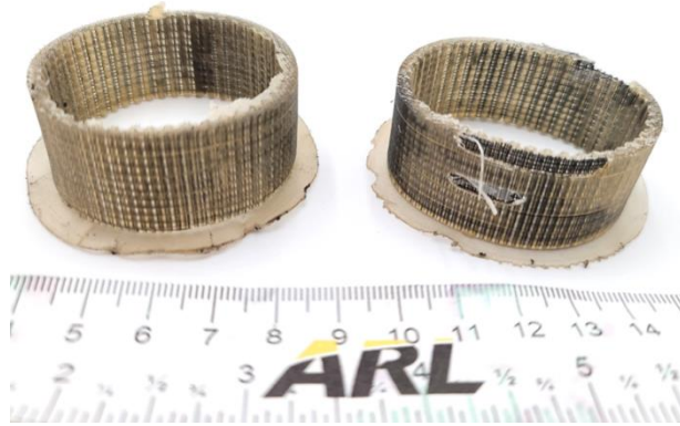
Figure 9. Five-belt stack extracted from PLA mold (left) and from PLA mold coated with WD-40 (right).
