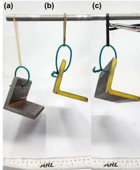
Figure 11. Static belt testing. (a) Belt fabricated without fiber reinforcement, (b) fabricated urethane belt with fiberglass reinforcement, and (c) benchmark belt with fiberglass reinforcement.
