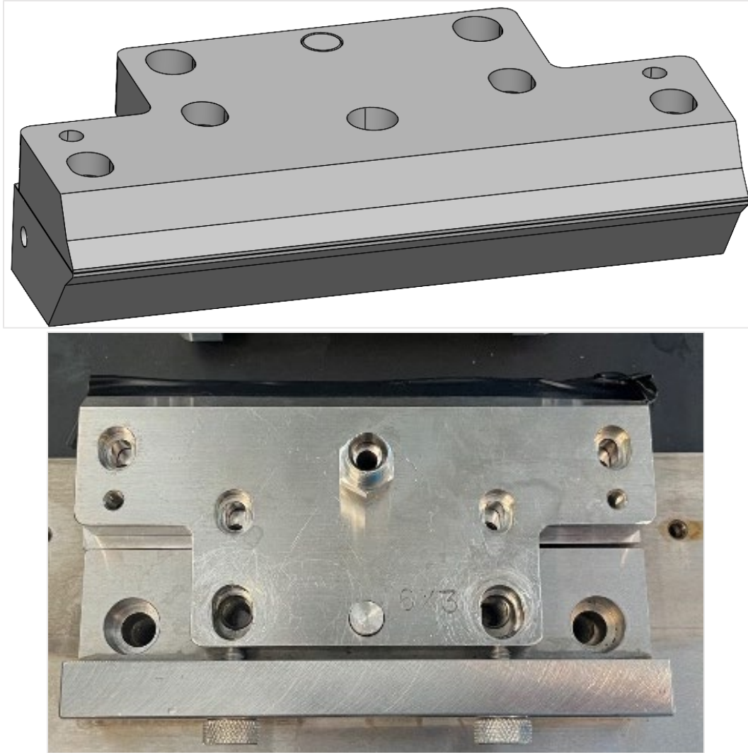
Figure 2. Model (top) and photograph (bottom) of the slot die.
