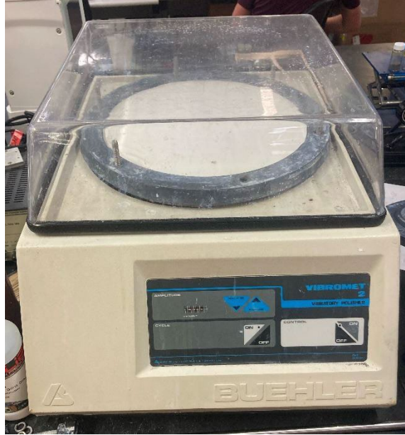
Figure 8. VibroMet 2 automatic polisher used for final polishing steps.
