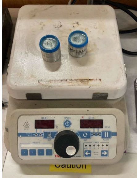
Figure 2. Hot plate setup used for heating Crystalbond on an aluminum puck mount.
