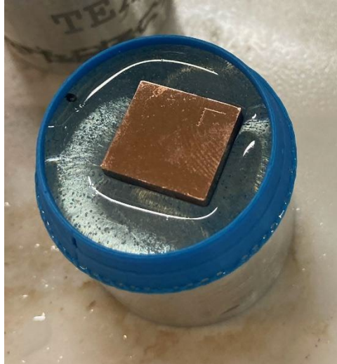
Figure 5. Overhead view of molten Crystalbond surrounding a copper specimen prior to cooling.
