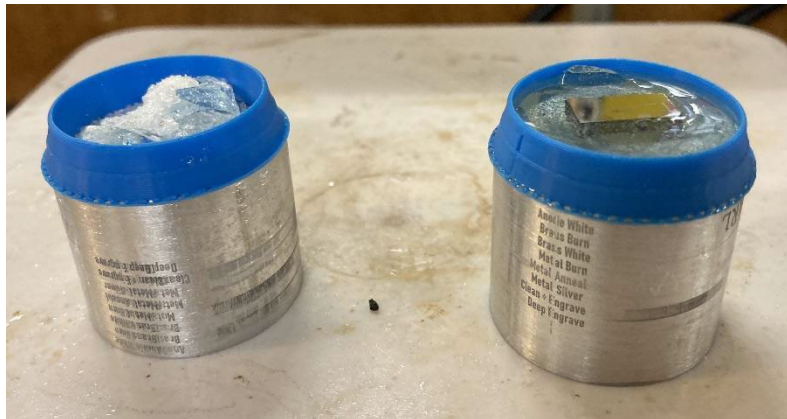
Figure 4. Sample showing solid Crystalbond shards portioned into a retaining ring (left) and a mounted specimen prior to cooling (right).
