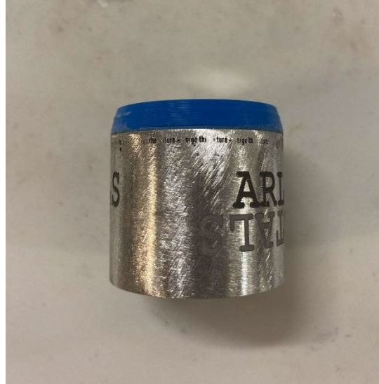
Figure 1. Example of proper fitment for a 3D-printed Crystalbond retaining ring mounted onto an aluminum puck.
