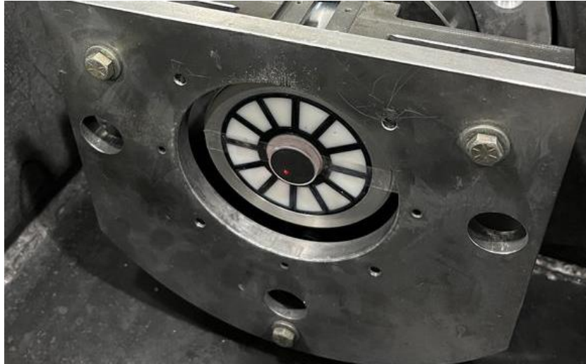
Figure 1. Loaded sabot with alignment mirror taped to front face.
