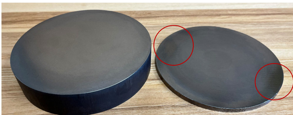
Figure 4. New potting plate (left) next to older plate (right). The circled regions on the old plate are low spots on the surface caused by plate bending and appear darker due to not making contact with the lapping plate during refinishing.
