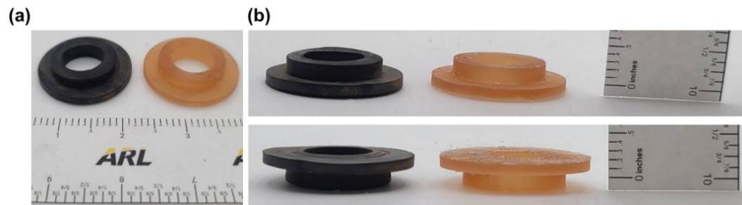
Figure 5. Comparison of OEM (black) and cast gladhand seal: (a) angled and (b) side views.
