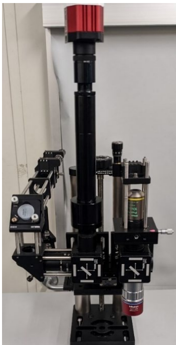
Fig. 11 PL microscope with conjugate image planes for TMD studies
