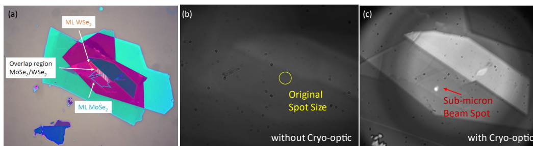
Fig. 12 (a) An optical microscopic image of the stacked MoSe 2 /WSe 2 heterostructure sample from Professor Philip Kim's group at Harvard, with different stacked regions labeled and colored for clarity. (b) Previous image of sample in PL apparatus with \sim 2\text{-}\mu\text{m} spot size superimposed. (c) New image of sample in apparatus with improved image quality and submicron beam spot size that results in better spatial resolution. Improvements in image clarity and resolution, and excitation laser spot size were primarily achieved through installation of a cryo-optic objective located inside the cryostat chamber.
