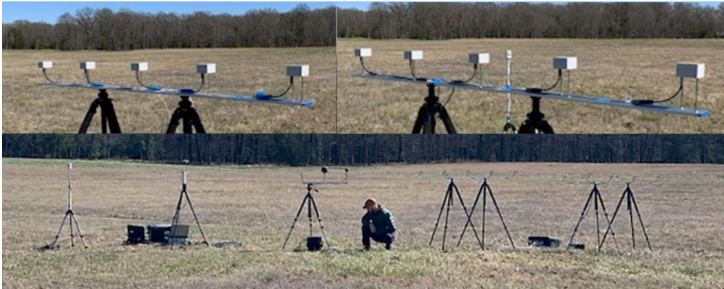
Figure 3. The experimental setup. Inserts at top show closer images of the enclosures and mounting bars.
