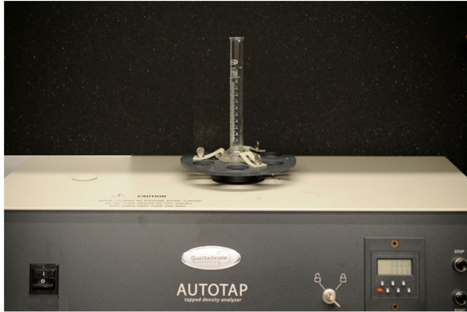
Figure 7. Tap densometer with 10-mL glass graduated cylinder. Measurements were typically initiated on powder volumes of about 8 mL.
