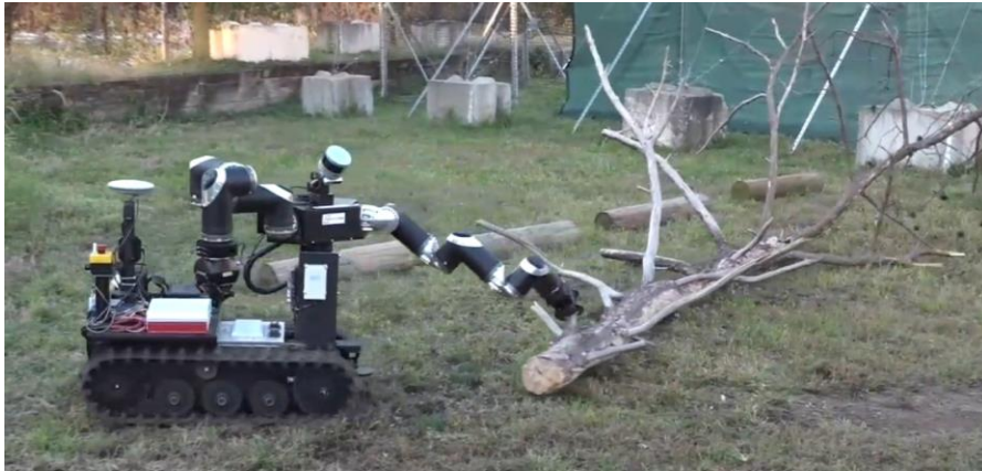
Figure 1. RoMan bimanual robot autonomously removing a tree from a notional roadway. 5
