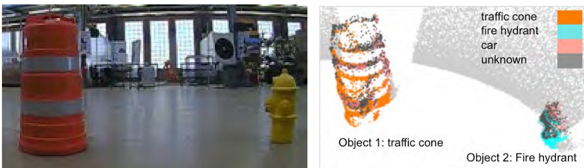
Figure 3. Example of object detection with lidar fusion, with actual objects (left) and labeled point cloud images (right).
