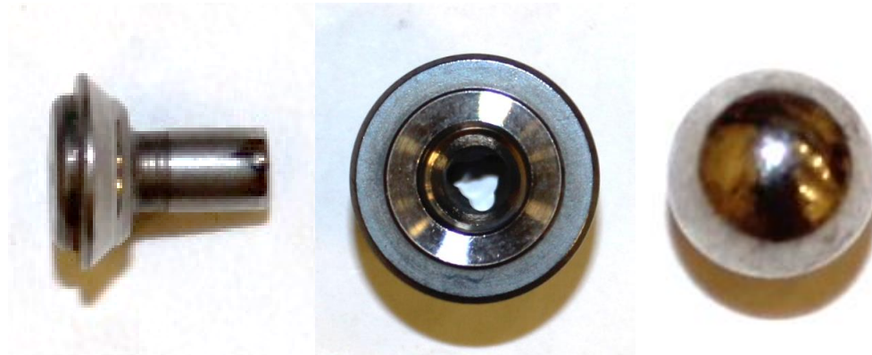
Figure 69. Inlet suction and outlet check valves from pump 5 (fuel 2, 1200 h). Left, inlet suction valve; bottom center, inlet valve seat; right, check valve ball.
