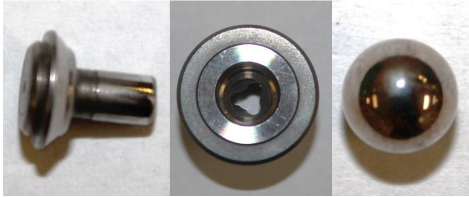
Figure 67. Inlet suction and outlet check valves from pump 4 (fuel 2, 476 h). Left, inlet suction valve; bottom center, inlet valve seat; right, check valve ball.
