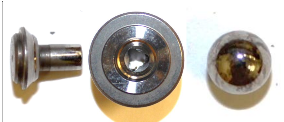
Figure 63. Inlet suction and outlet check valves from pump 2 (fuel 1, 1052 h). Left, inlet suction valve; bottom center, inlet valve seat; right, check valve ball.
