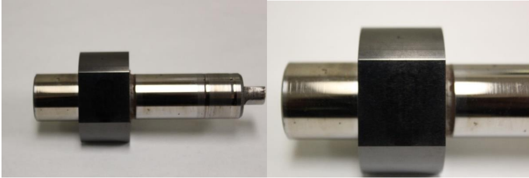
Figure 19. Camshaft and cam ring from pump 5 (fuel 2, 1200 h).
