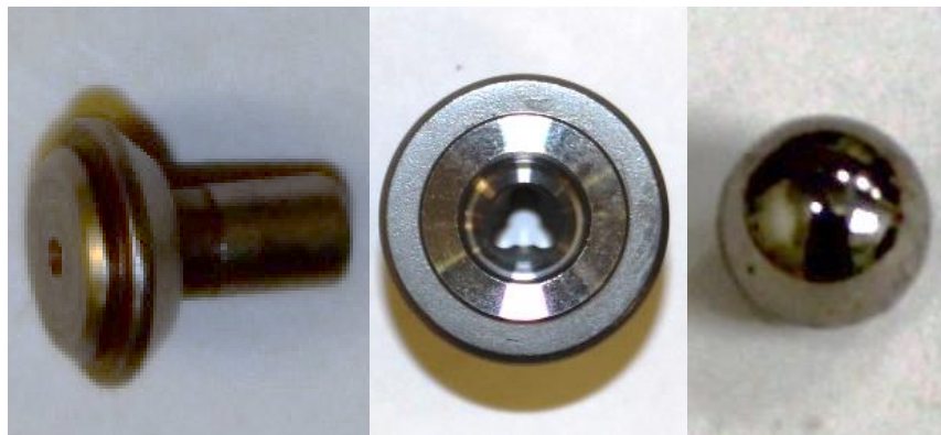
Figure 60. Inlet suction and outlet check valves from pump 1 (pristine, 0 h). Left, inlet suction valve; bottom center, inlet valve seat; right, check valve ball.
