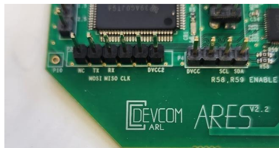
Figure 5. The six-pin header for SPI or UART communication and four-pin connector for I2C communication are shown. Both can be used to send or receive data from either onboard processor.
