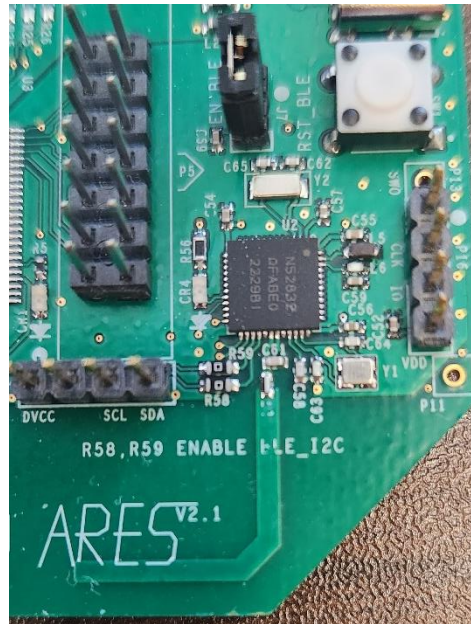
Figure 6. Back-end processing section. It includes nRF52 to read data via SPI or I2C, a 2.45-GHz PCB antenna to transmit processed data over BLE, a reset button, and a four-wire programming interface.
