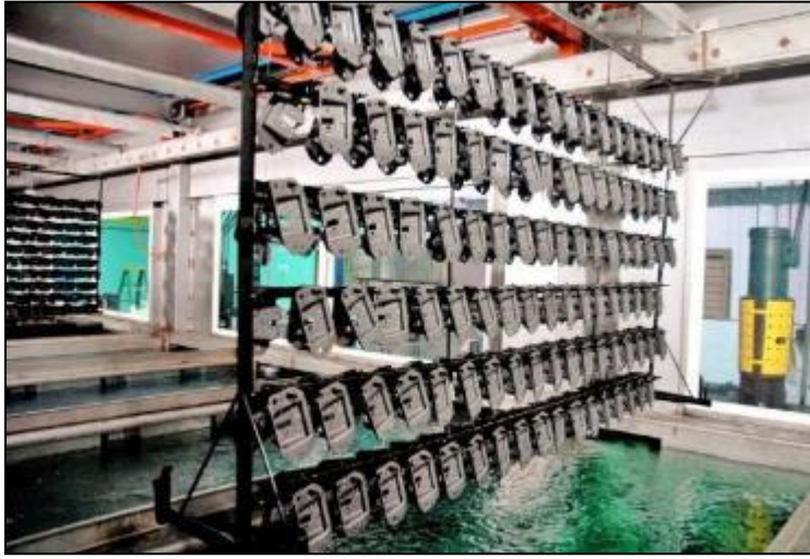
Figure 6. Parts progressing through an e-coat system at Blue Grass Plating in Richmond, Kentucky. The scale of an e-coat line must be matched to part size and throughput to minimize cost and footprint while maximizing bath stability (photo courtesy of Therma-Tron-X, Inc.).
