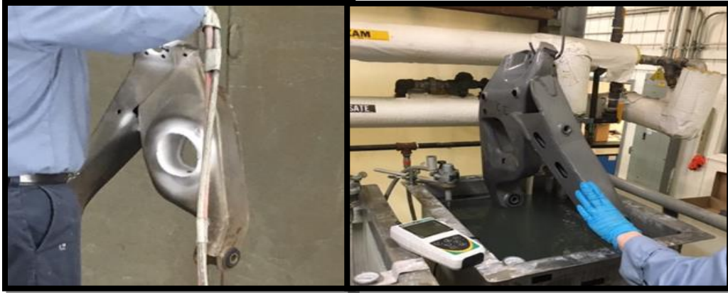
Figure ES-2. Toll coating of MIL-DTL-53022 primer at Aalberts Surface Technologies (left) and e-coat at PPG's Euclid facility (right).
