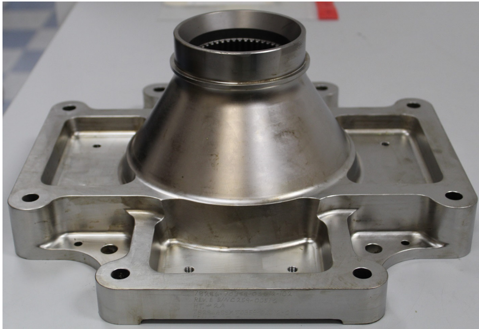
Figure 12. UH-60 tail rotor gearbox following ablation.
