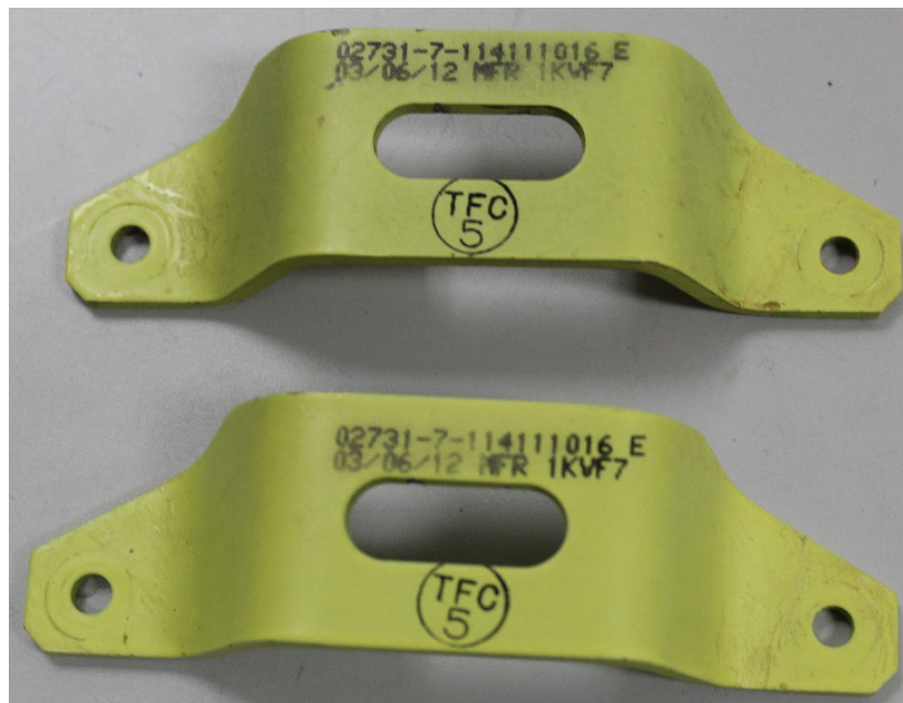
Figure 9. AH-64 main rotor head nut retention brackets, as received.
