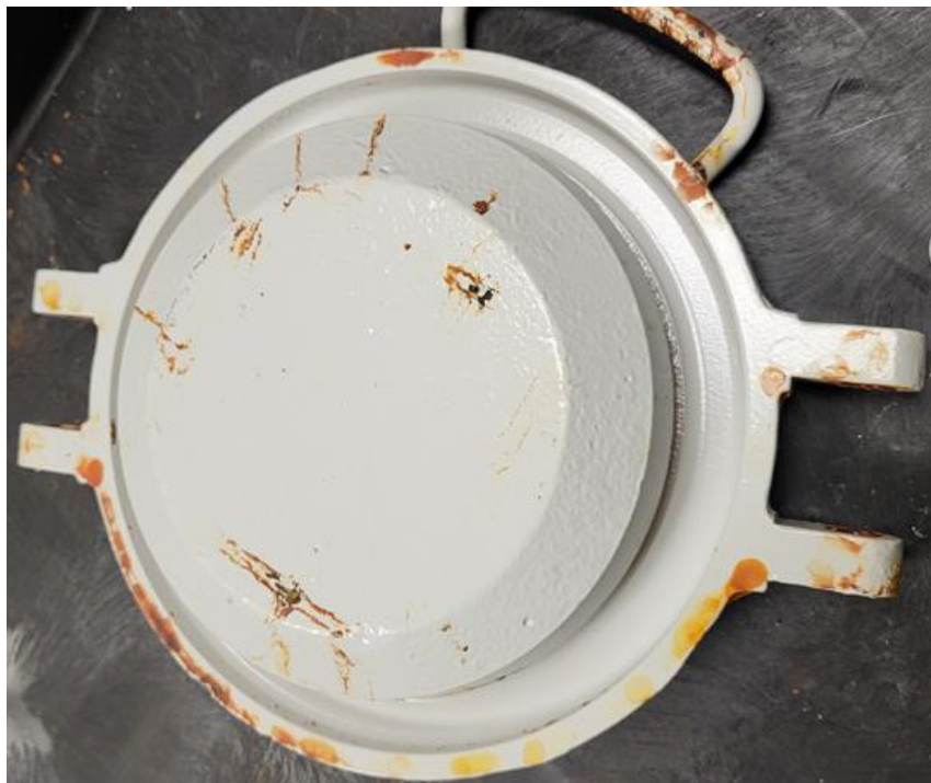
Figure 19. Steel M1 fuel cap at 1008 h (ASTM B117) (bottom).
