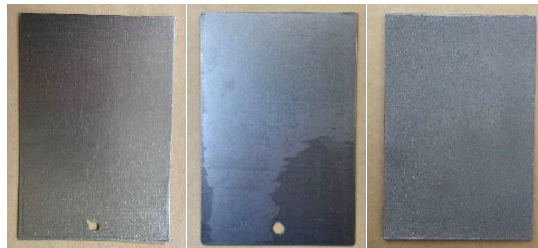
Figure 2. Representative ablated samples (left to right: AA2024, CRS, and HHA).
