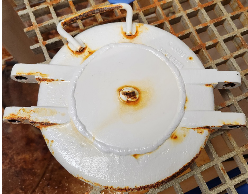
Figure 18. Steel M1 fuel cap at 1008 h (ASTM B117) (top).
