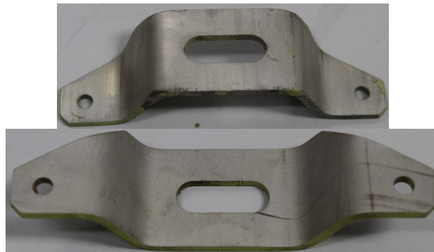
Figure 14. AH-64 main rotor head nut retention brackets following ablation.
