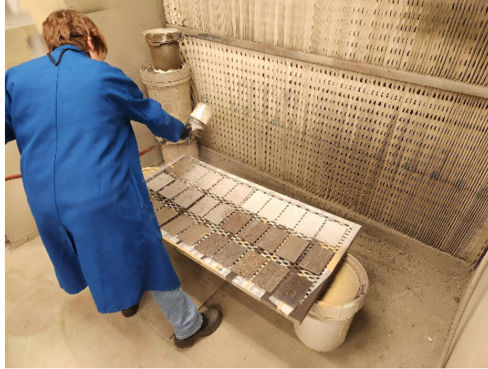
Figure 1. Test panels being coated with primer.
