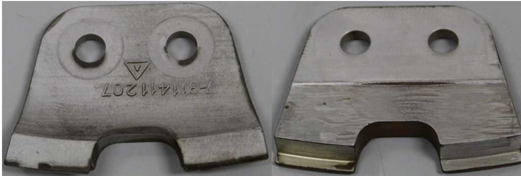
Figure 13. AH-64 main rotor head bearing retainers following ablation.
