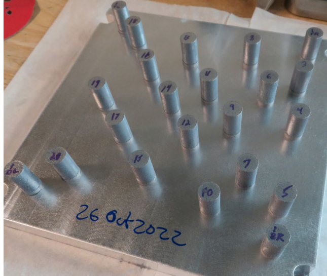
Figure 2. Metallography cylinders as printed, before removal from support structures and build plate.
