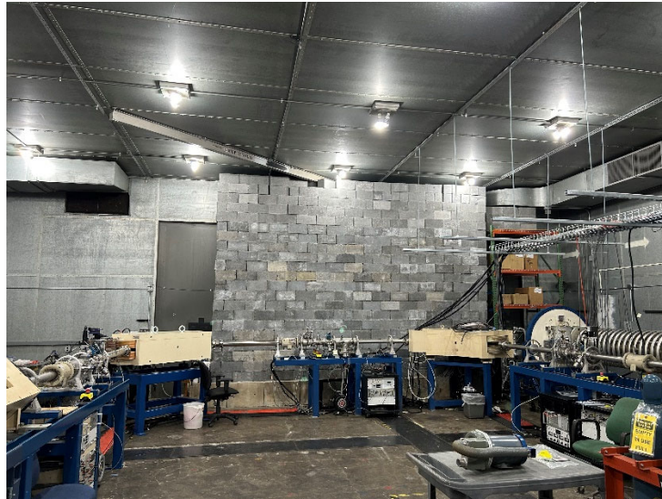
Figure 6. Inside the Test Cell looking in the direction of the Bay Wall. A ventilation supply duct and return vent structure are in the top left part of the Bay Wall that occupies a left passthrough, whereas a similar structure in the top right part of the Bay Wall is obstructed by a set of concrete blocks. A similar block structure was in front of the left return vent only, but it had to be removed during installation of the Pelletron beamline components. The large concrete Block Wall was erected before operation of the electron linacs to reduce radiation passing through the Dimple Plate. The Pelletron beamline carries ions (right) toward the Bay Wall, turns them left past the Block Wall, then again turns the ions away from the Bay Wall toward the camera.
