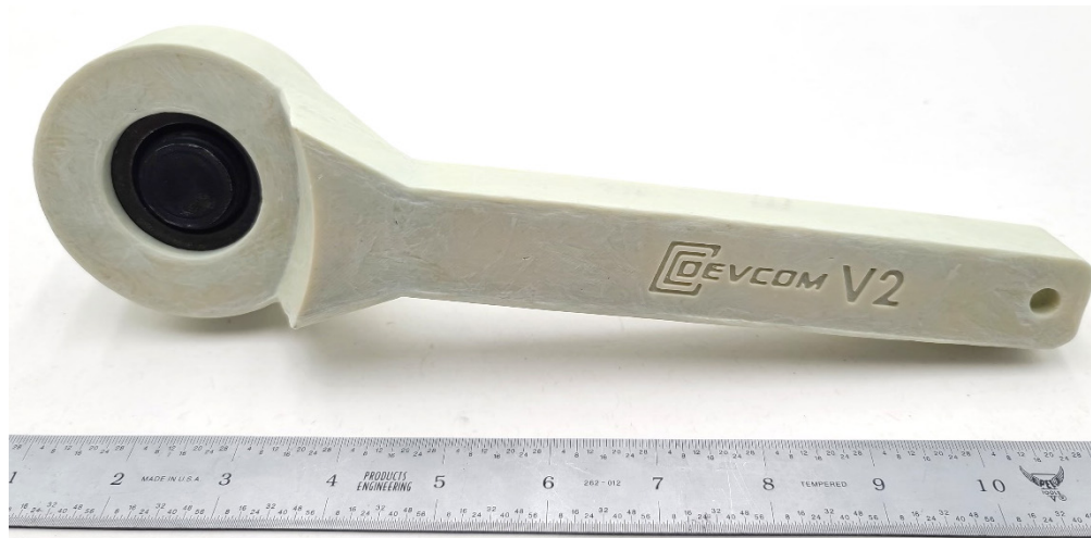
Figure 8. Fabricated electrically insulating wrench with DEVCOM logo on the handle.
