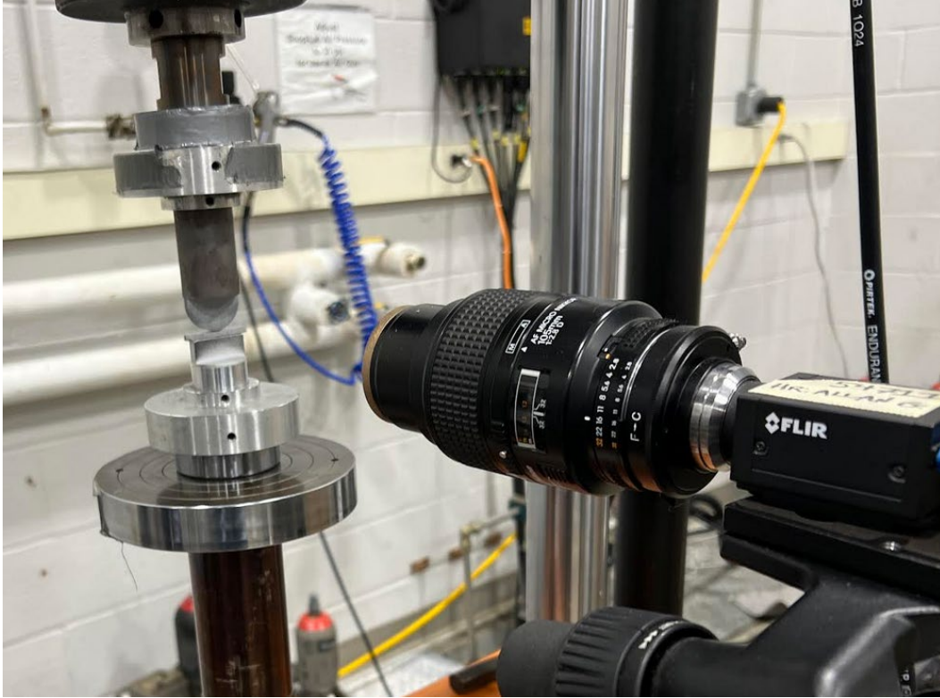
Figure 6. Loading setup for low loading rate experiments, pictured with blunt geometry indenter.
