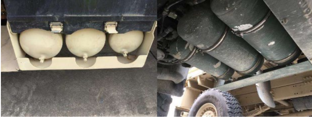
Figure B-9. Hydraulic and air tanks.
