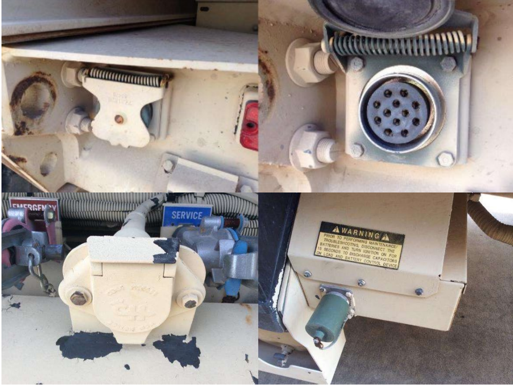
Figure B-3. Electrical connectors and components.
