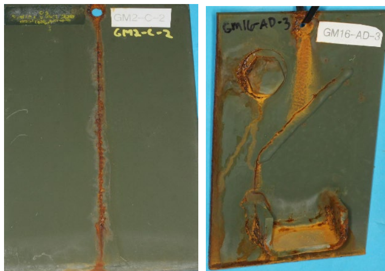
Figure 7. Scribe panel vs. complex panel, 40 cycles GMW14872, 5 CARC.
