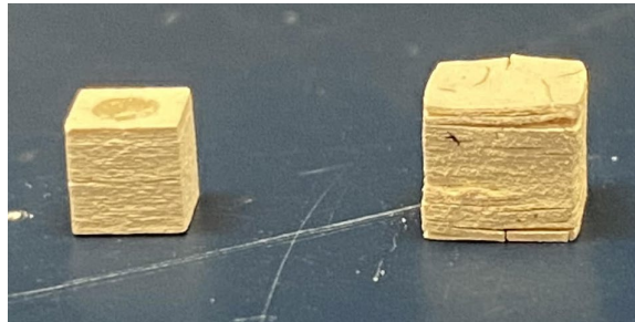
Figure 2. Images of 3D-printed GDC samples after debinding. The sample processed using the optimized, temperature-controlled debinding schedule (left) substantially reduced cracking and minimal layer distortion, whereas the sample processed without staged temperature control (right) shows pronounced cracking and interlayer deformation.
