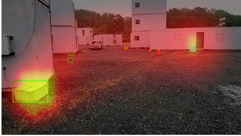
Figure 3. Example POV video frame. Green bounding boxes indicate object detection output from Grounding DINO. Overlaid heat map indicates attentional priorities assigned by RAGNAROC.
