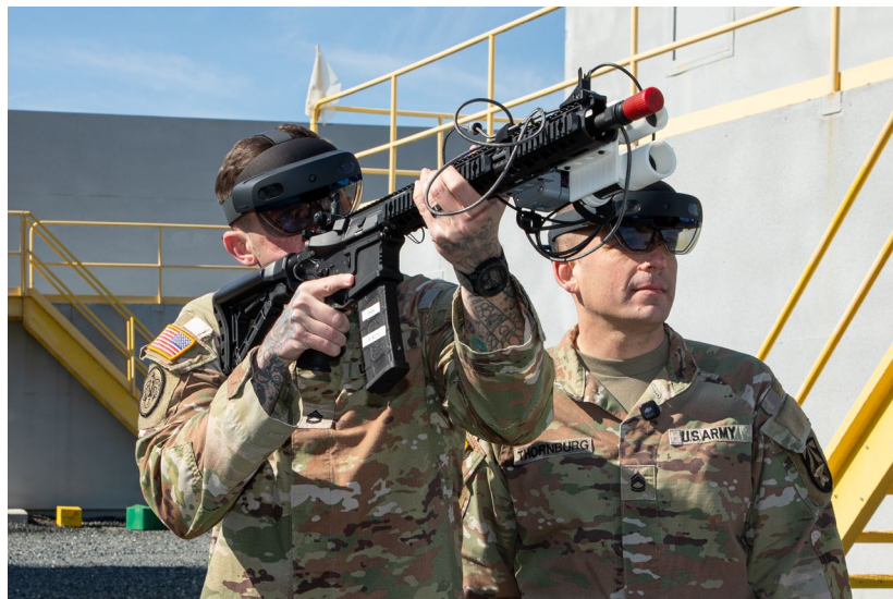
Figure 5. Instrumented rifle with video, IMU, GPS, and magnetometer.
