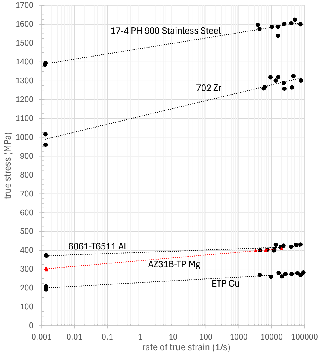
Figure 13. Rate effect for all materials. The magnesium data using 0.7- and 0.35-mm samples has been omitted due to the inconsistency with the larger samples.
