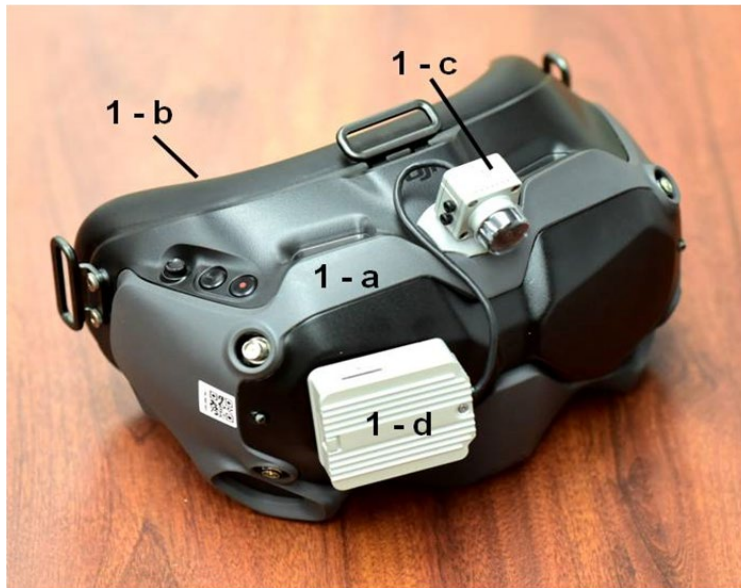
Figure 1. An oblique view of the camera device configured for small camera-to-goggles separations.
