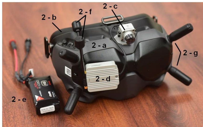
Figure 2. An oblique view of the device configured with antennas to allow for the camera (2-c) and transceiver (2-d) to be separated from the goggles (2-a) and placed hundreds of meters away. The transceiver battery (2-e) is also shown.
