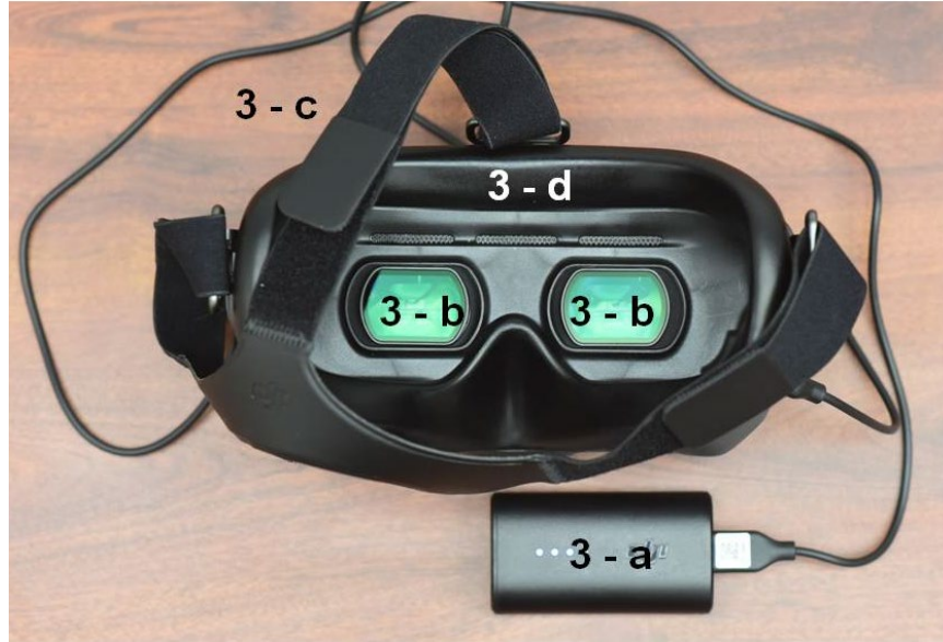
Figure 3. A rear view of the device showing the mounting straps (3-c), the LED displays (3-b), the face seal (3-d), and the goggle battery (3-a).
