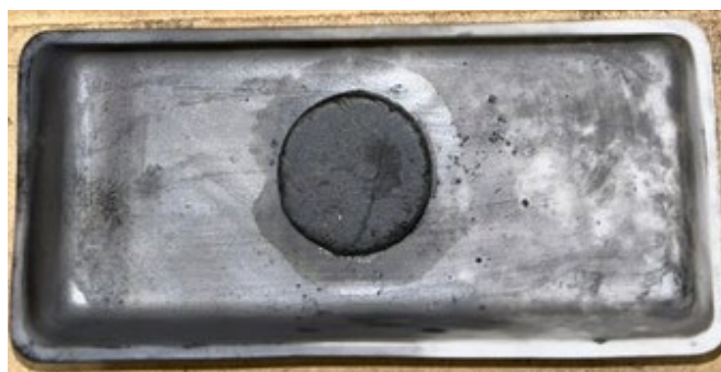
Figure 7. Image of a 1-inch puck of ceramic after infiltration with SMP-10 and heat treatment to 300 °C. Note the ring on the crucible around the base of the puck due to leakage of the polymer out of the puck.
