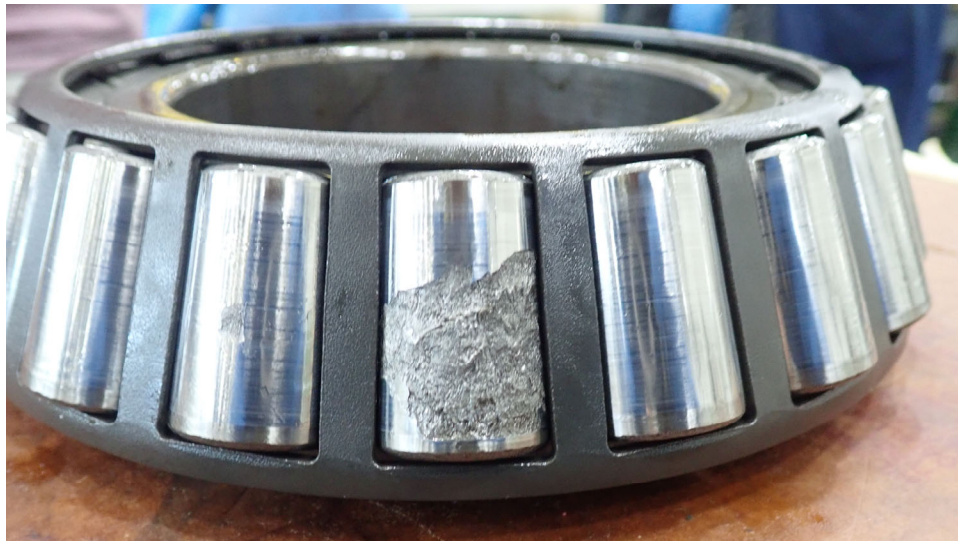
Figure 10. PI3 bearing damage found during overhaul.
