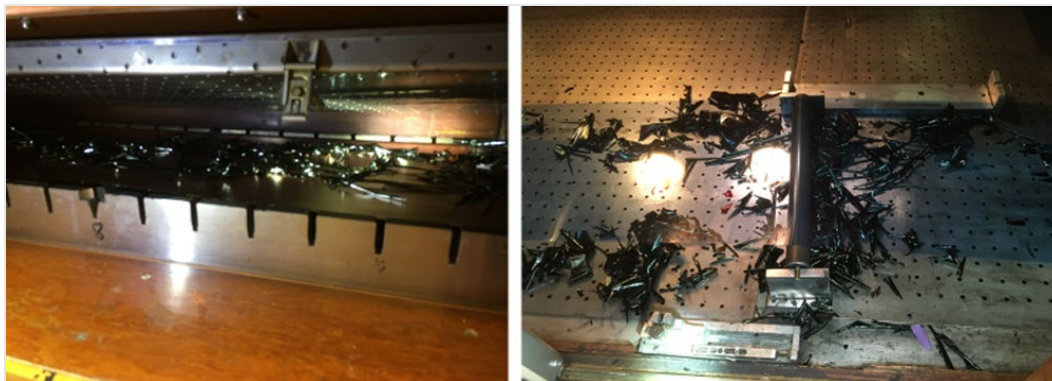
Figure 11. Result of the coating (shown in Figure 10) moving through the dryer section of the RC5. The coating rapidly delaminated and shredded itself. This may have resulted from high RH, high dryer temperature, issues with poor support adhesion, or any combination of these causes.
