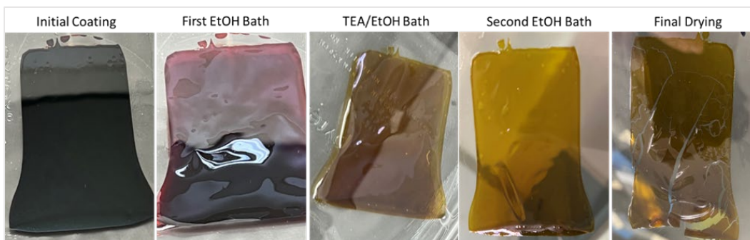
Figure 8. Images from left to right show the progression of monomer coating ID 20220407-A as it goes through the different stages related to its neutralization. Note: This coating remained as seen in the leftmost image for over 40 min under low RH conditions without any of the issues observed with similar coatings held at ambient conditions with higher RH.
