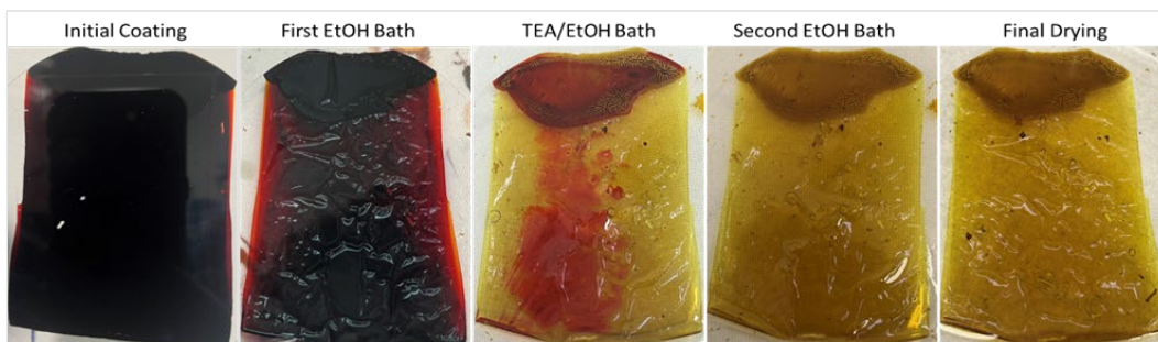
Figure 7. Images from left to right show the progression of monomer coating ID 20220330-A as it goes through the different stages related to its neutralization. This coating was a replicate of the ID 20220328-A coating.
