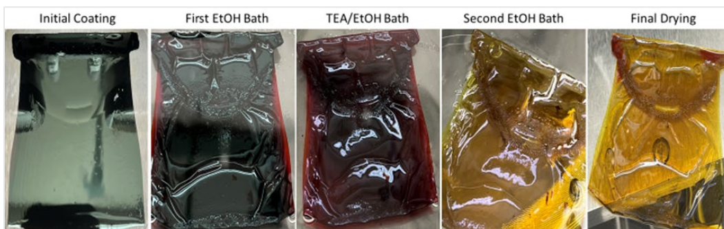
Figure 6. Images from left to right show the progression of monomer coating ID 20220328-A as it goes through the different stages related to its neutralization. Note: “Fingerprinting” seems to appear in regions where flow is inconsistent and fluid has flowed over an already coated region.
