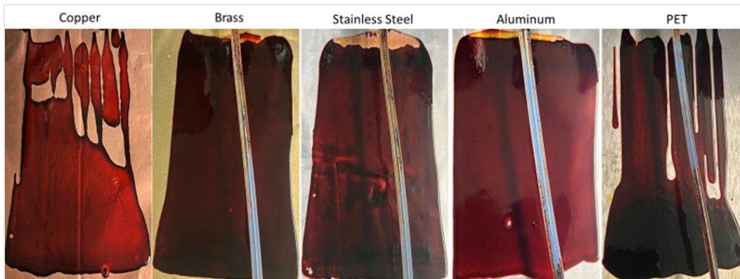
Figure 12. The initial coating images for the support study intended to give data on whether the shredding/spontaneous delamination was affected by the support.
