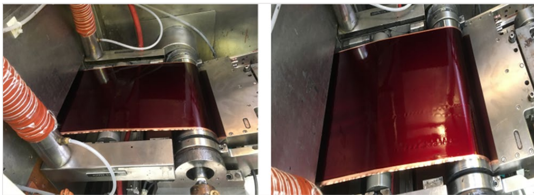
Figure 10. Examples of visually good coatings at the slot die. They are coated onto copper support and display no break lines or pull through with good edge control, indicating that the coating thickness is as expected and there is no lost material.
