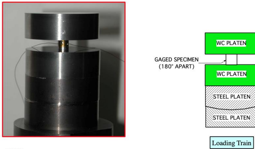
Fig. 3 Photo and schematic of the LR and IR experimental setup showing the loading axis comprising the strain-gaged specimen, WC platens, and spherical steel platens
