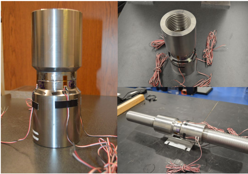
Fig. 10 Strain gauge configuration showing placement at the bond line in 90° intervals
