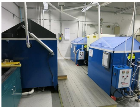
Fig. 2 Neutral salt fog corrosion chambers used for testing
