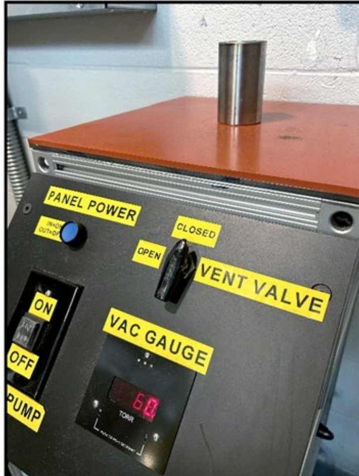
Fig. 3 Vessel leak checker with HIP can during testing
