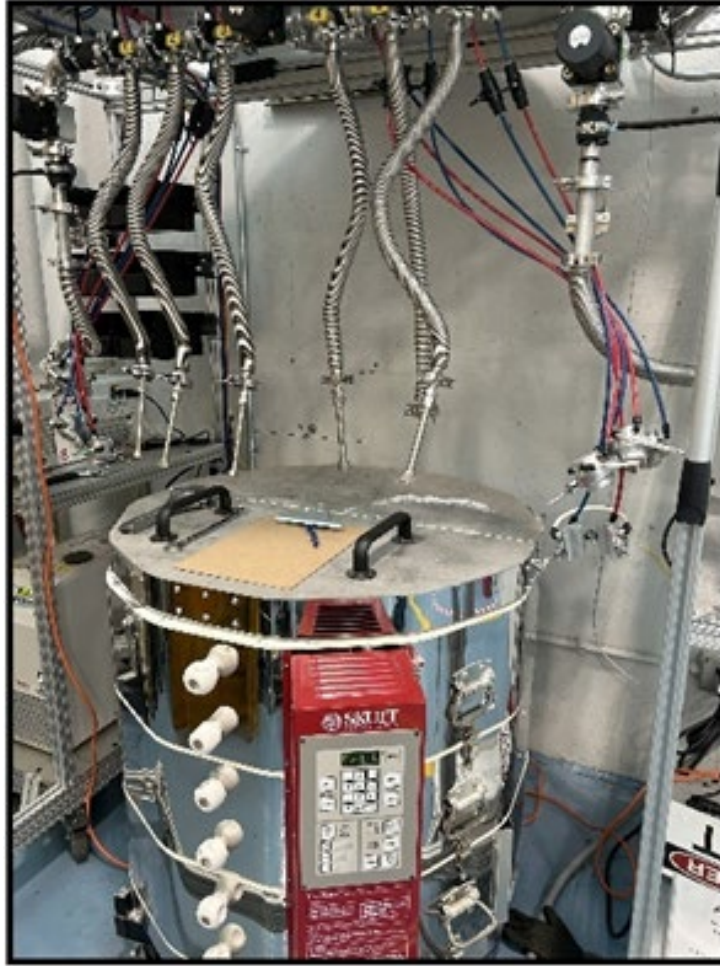
Fig. 5 Bakeout furnace with manifold for multiple HIP can vessels
