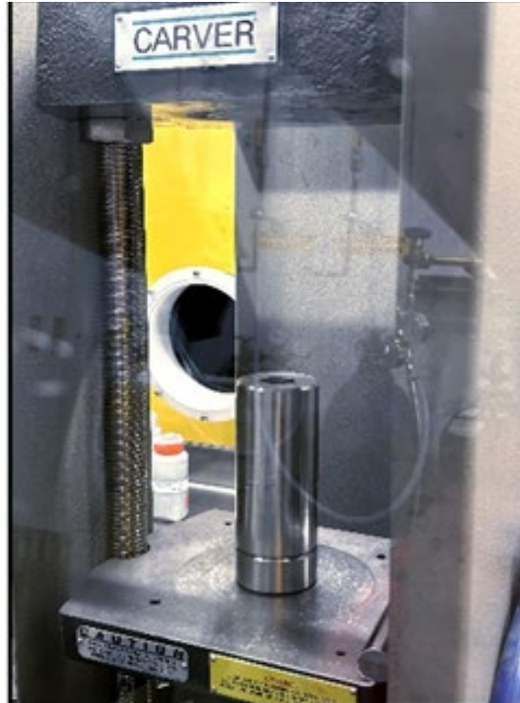
Fig. 7 Carver press inside the glovebox
