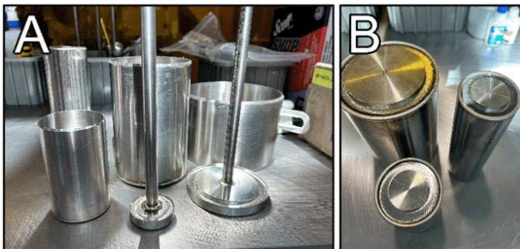
Fig. 2 A variety of HIP vessels before powder loading, as well as stems and caps. The 60° chamfers can also be seen (A), and the welded ends of the HIP vessels before leak testing (B).
