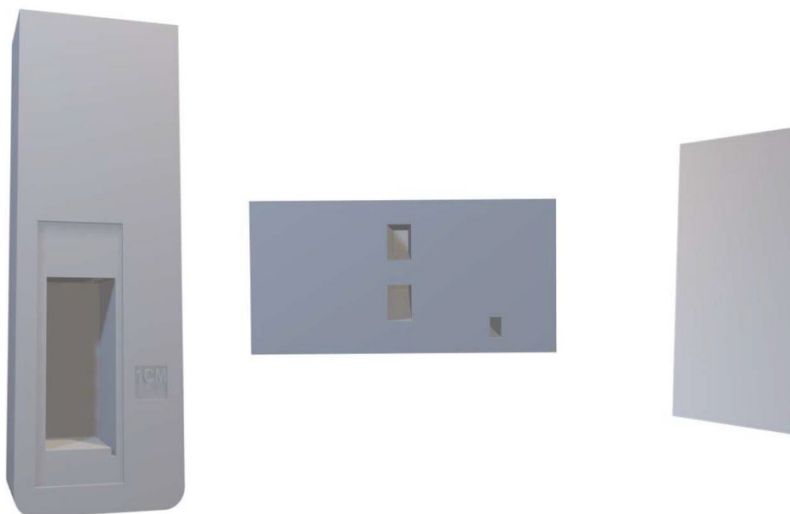
Fig. 10 Electrolyte Mount 4-3 (left); top view (middle); matryoshka piece (right)
