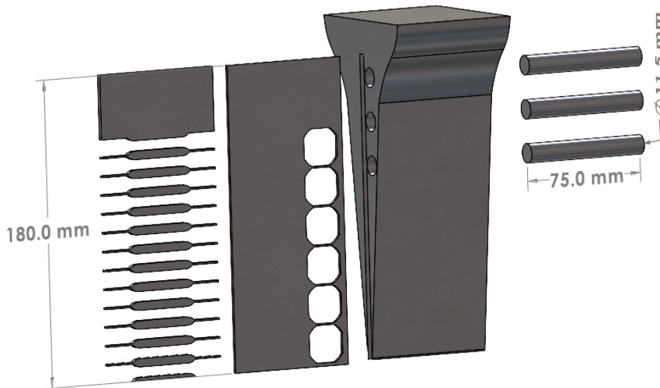
Fig. 2 Exploded view of samples sectioned from the wedge castings
