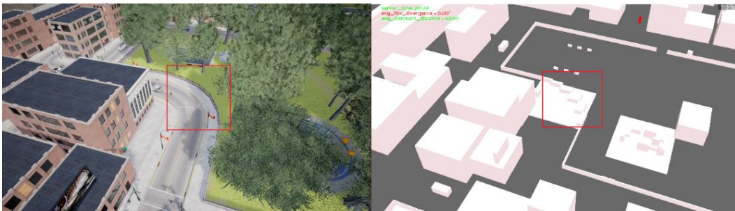
Fig. B-11 A side-by-side comparison demonstrating the spatial fidelity limitation. On the left, a curved section of wall in the commander's interface world. On the right, the tvp3d representation of the actors. Because the curve lies diagonal to the x and y world axes, the smallest axes-parallel envelope becomes wider along both the x and y axes. While the straight sections of wall are axes-aligned and accurately represented, the curved section's size becomes inflated.
