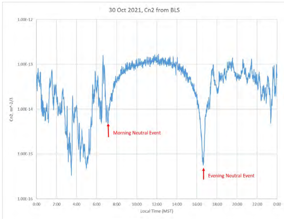
Fig. 20 NATurE Phase 1 BLS measurements, 30 Oct 21
