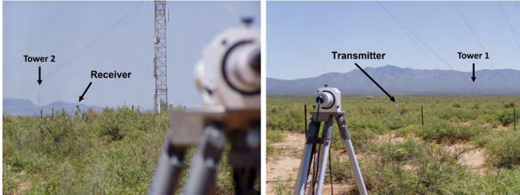
Fig. 5 Phase 1 SLS 40A setup at MSA Tower 36; view from SLS transmitter (left) and view from SLS receiver (right)
